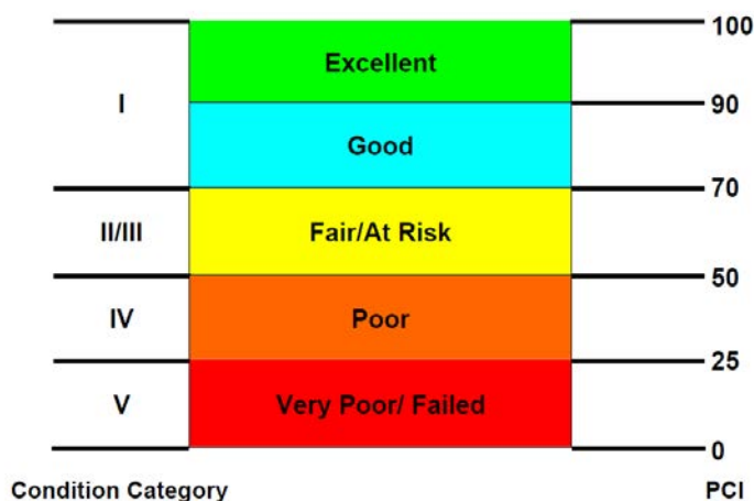
Figure 3. Pavement Condition Index Rating Chart
