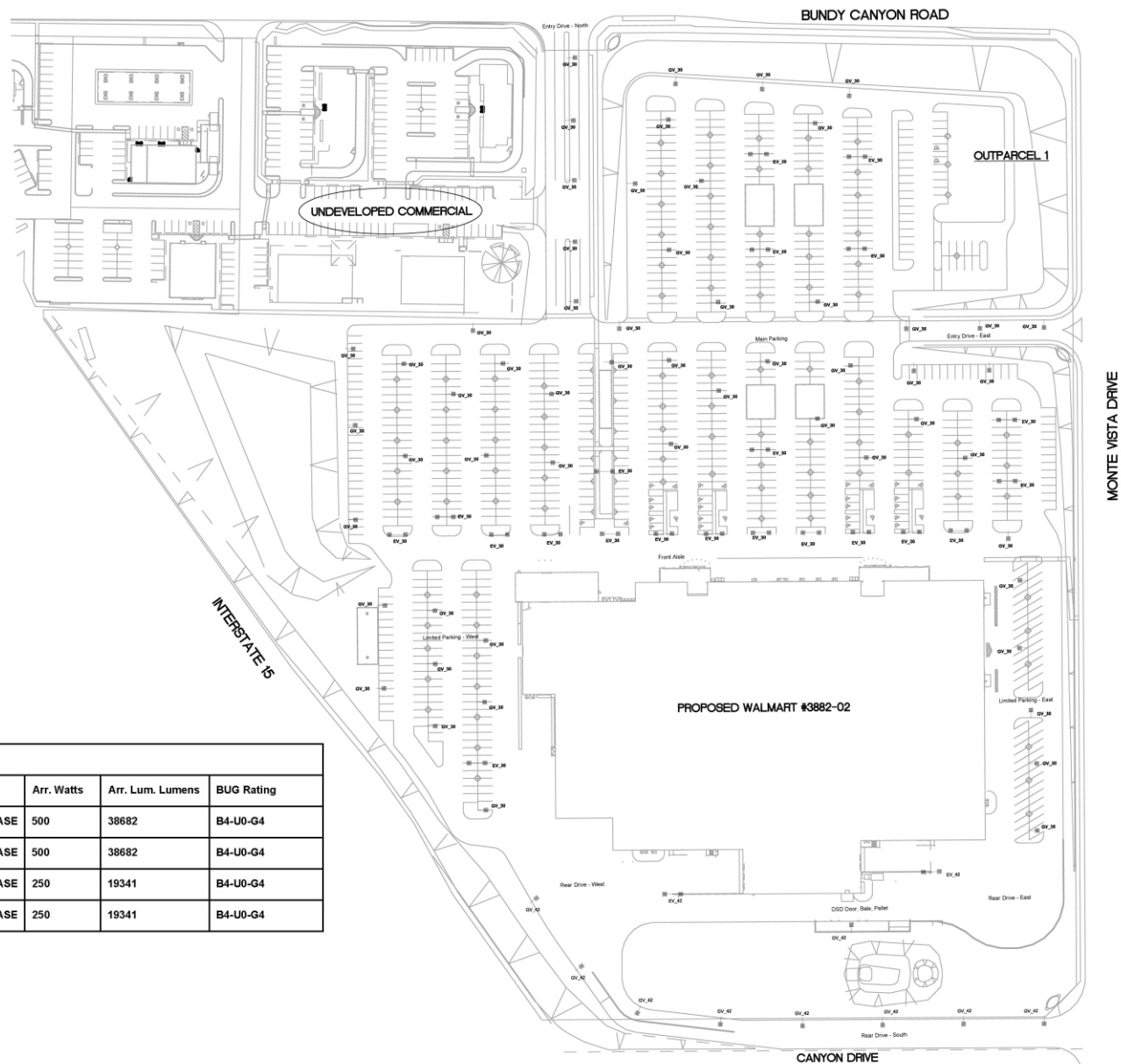
Figure 3.4-12 Lighting Plan - Luminaire Locations
