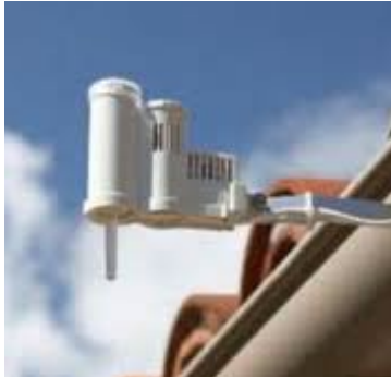
Sensor automatically adjusts controller daily run times based on local climate conditions to reduce water usage
