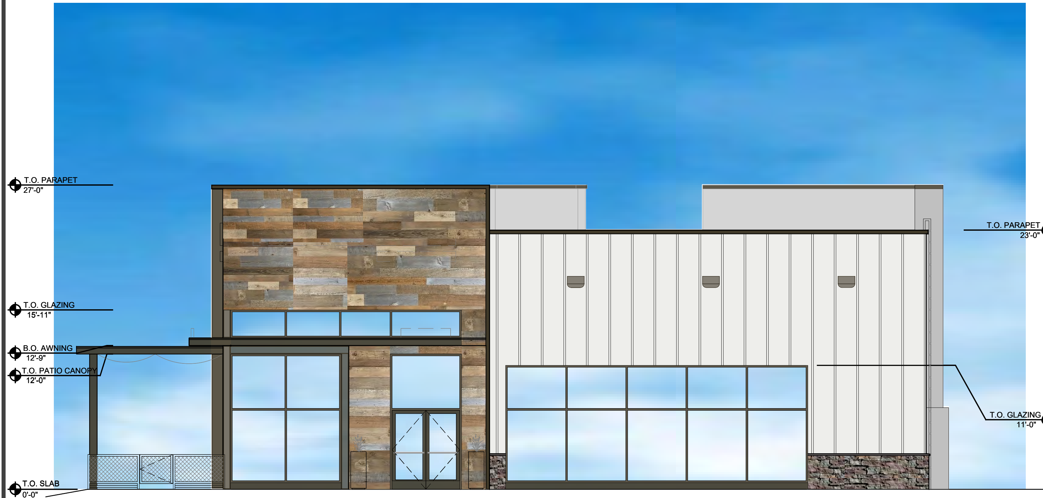
1 EXTERIOR NORTH ELEVATION A4.0 1/4" = 1'-0"
